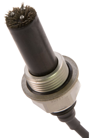
Sensor with debris attached
